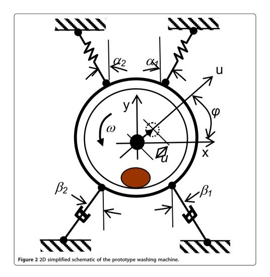
vibration to become more severe and hard to control. In the design of the suspension system for the tub assembly, the frequency range of the resonance in all directions should be as small as possible. From the above, it is easy to show that, by choosing  $\alpha_1 + \alpha_2 = 90^\circ$  and  $\beta_2 + \beta_2 = 90^\circ$ , Equation 1 can be simplified to yield
