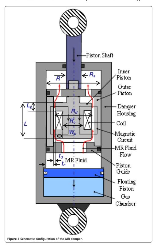
lower chambers. These chambers are fully filled with the MR fluid. As the piston moves, the MR fluid flows from one chamber to the other through the annular duct (orifice). The floating piston incorporated with a gas chamber functions as an accumulator to accommodate the piston shaft volume as it enters and leaves the fluid chamber.
