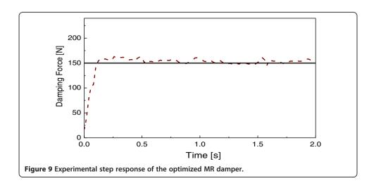
of the MR damper is measured on the downward motion of the shaft. In the figure, the solid line presents the calculated damping force while the dash line presents the measured one. The results also show that, at the steady state, the average damping force is around 157 N which is a little greater than the calculated one (150 N). The difference may result from friction which is not taken into account in the modeling of the damper.
