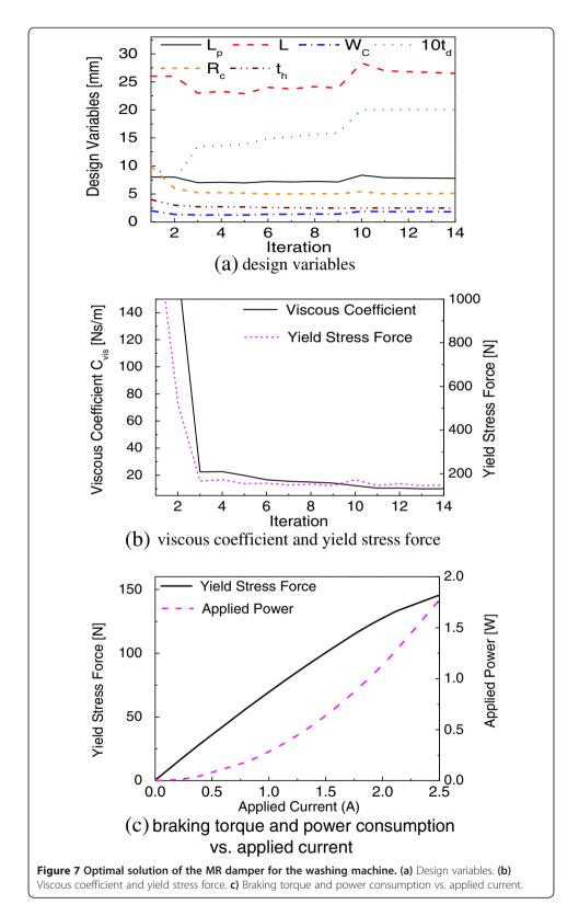
around 0.01 which is very small so that a very small transmissibility of vibration from the drum to the cabinet at high excitation frequency can be achieved. It is also observed from the figure that the yield stress force of the damper at the optimum is
