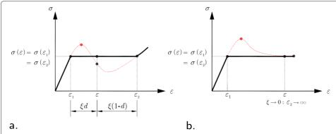
**Figure 4 Two micro-strains**  $\varepsilon_1$ ,  $\varepsilon_2$  **and the relaxed stress**  $\sigma$ . (a) A finite thickness of a micro-shear band. (b) A zero thickness of a micro-shear band.
