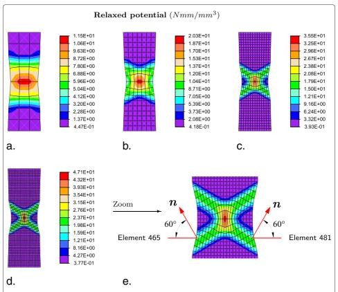
Figure 11 Example 2: comparison of different finite element meshes. Distribution of relaxed potential at v = 1.0 mm. (a) 24 MES elements. (b) 126 MES elements. (c) 504 MES elements. (d) 1,134 MES elements. (e) Orientation of shear bands at element 465 and element 481.
