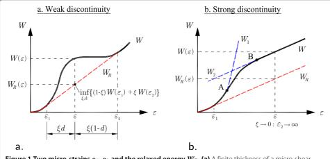
**Figure 1 Two micro-strains**  $\varepsilon_1$ ,  $\varepsilon_2$  **and the relaxed energy**  $W_R$ . **(a)** A finite thickness of a micro-shear band. **(b)** A zero thickness of a micro-shear band.
