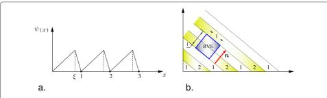
Figure 2 Laminates as special fluctuation fields  $\varphi$ . (a) Scalar function  $\Psi(x)$ . (b) Laminate of first order and representative volume element (RVE).
