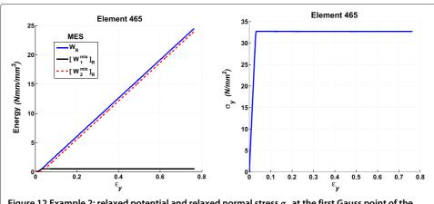
Figure 12 Example 2: relaxed potential and relaxed normal stress  $\sigma_y$  at the first Gauss point of the element 465.
