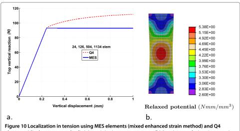
elements (displacement method). (a) Load-displacement response. (b) Distribution of relaxed potential.
